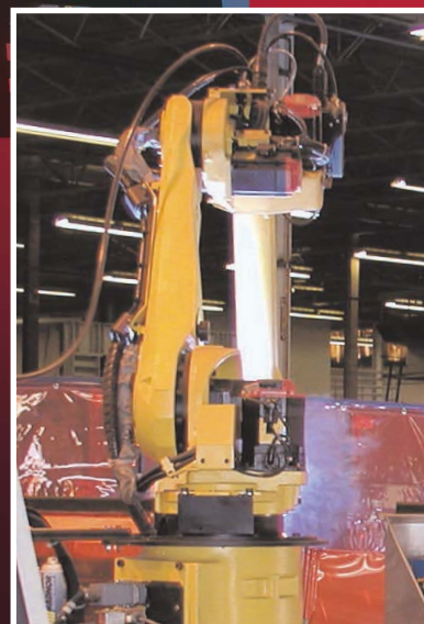
Six-axis robot performs full penetration welds.
